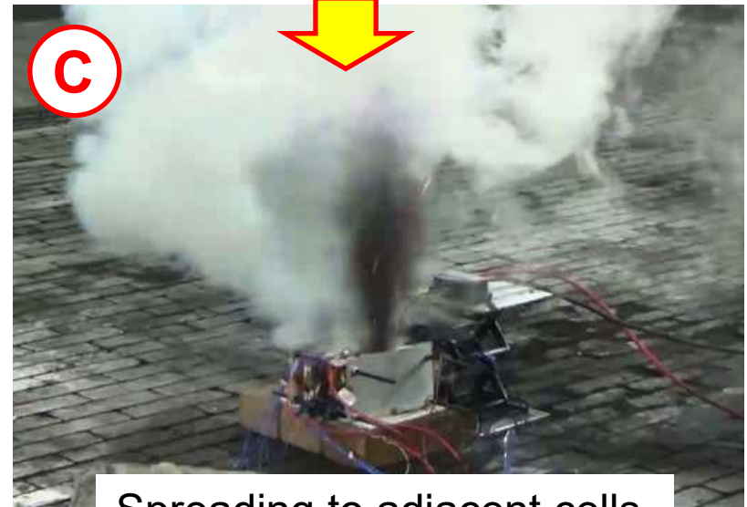
Spreading to adjacent cells (Thermal Propagation)
