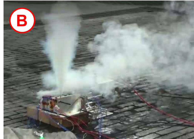
Outset of a cell thermal runaway
