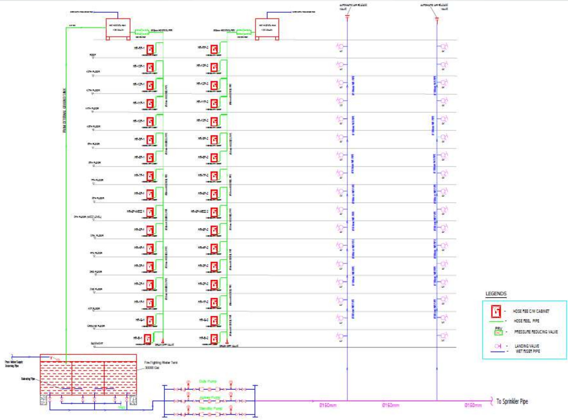
SCHEMATIC DIAGRAM OF FIRE HOSEREEL & WET RISER SYSTEM
