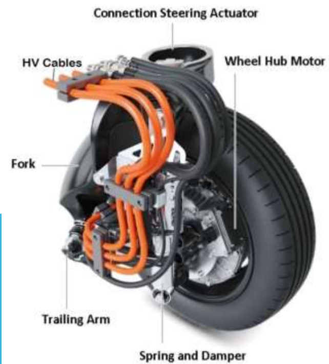
In Wheel Motor Assembly
