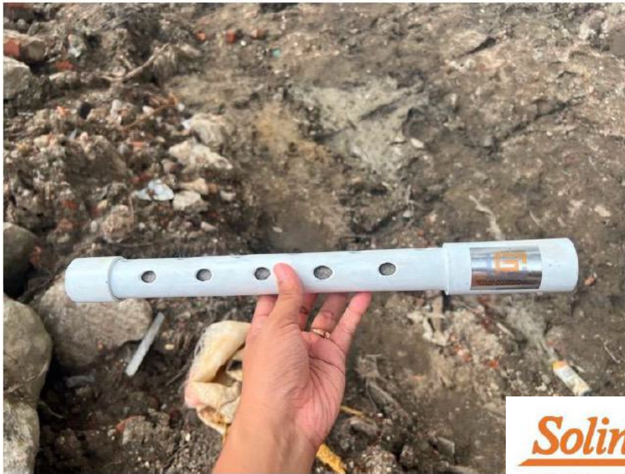
Figure 6: Casagrande Piezometer & Water Level Monitoring
