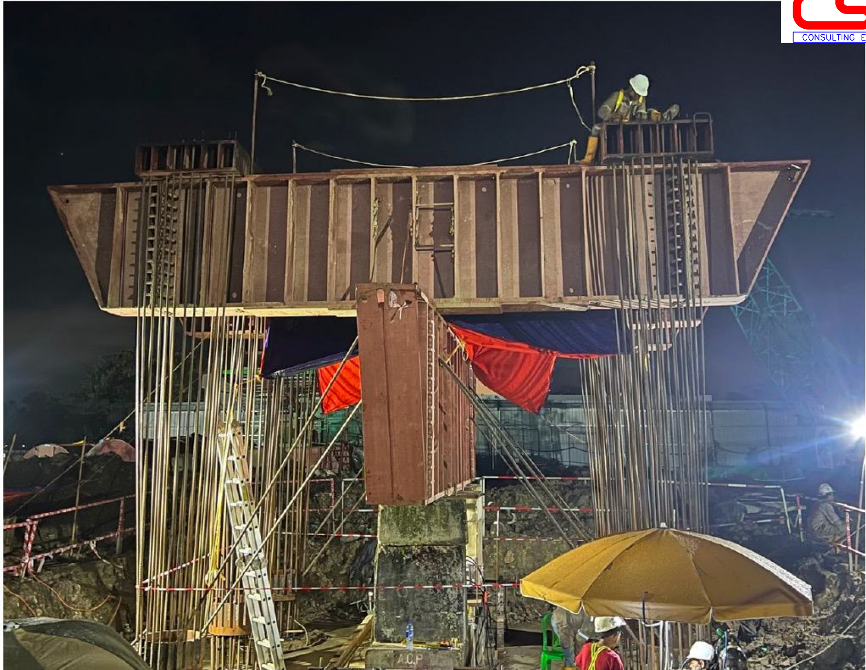
Figure F1: ULT Test Inverted Beam System Setup
