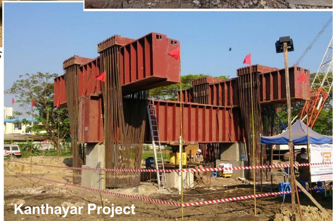
STATIC PILE LOAD TEST WITH INVERTED BEAM SYSTEM
