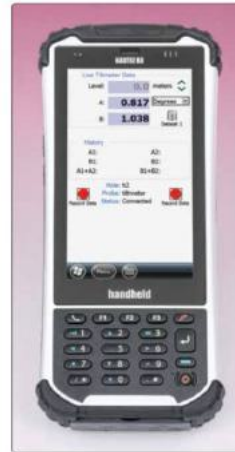
• Model PPC-2 Field PC showing a Live Tiltmeter Data reading screen shot.
