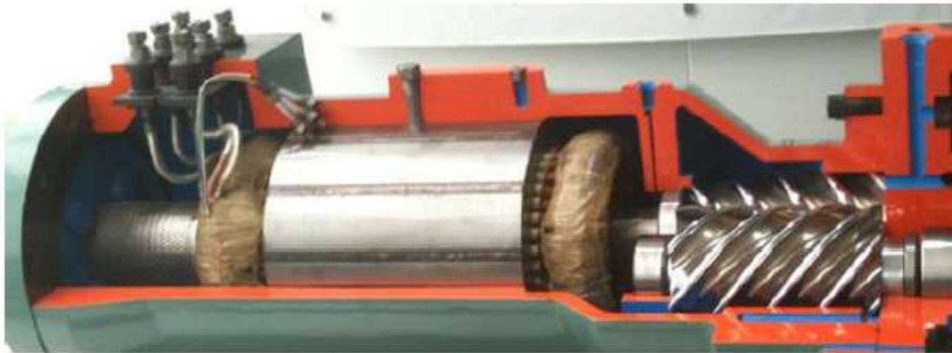
Figure 1.5 Sectional view of screw compressor
