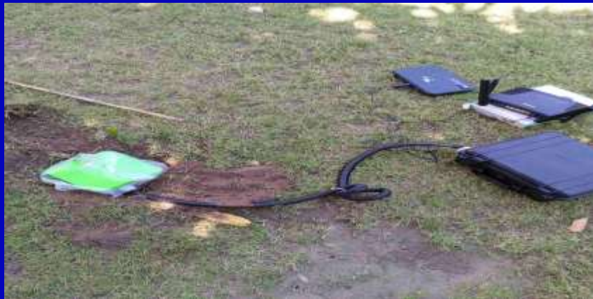
Microtremor survey (single) at FMI City
