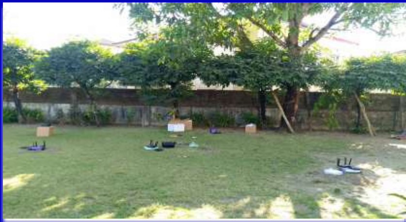
Microtremor survey (array) at FMI City
