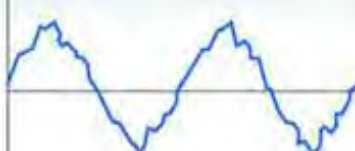
12-pulse system with Standard AC drive
