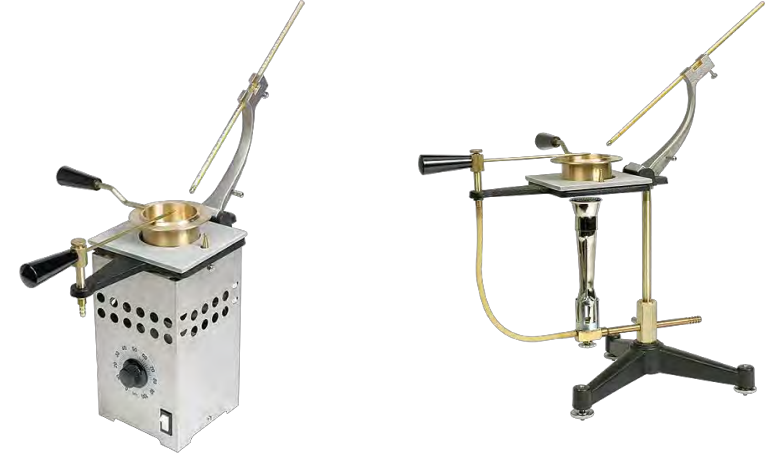
Cleveland Flash and Fire Point Tester
