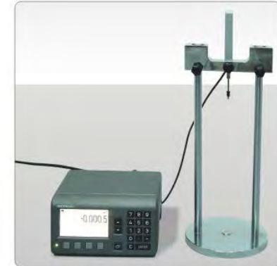
UTCM-0038 Length Comparator with Heidenhain Length Measuring Sensor
