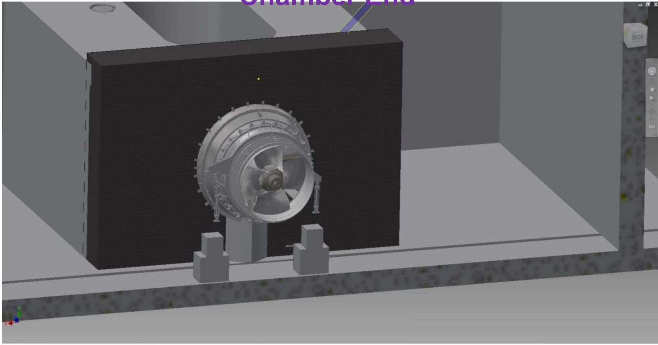
Fig. 36: Pit Type HFK Front View at Runner Chamber End
