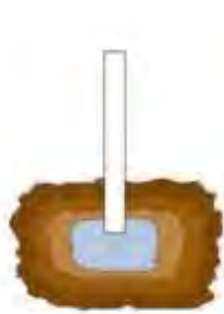
Compaction Grout (Displacement)
