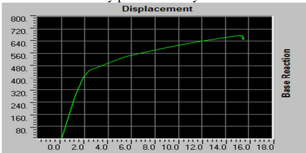
Fig-5, Case-1, Pushover curve for Displacement and base shear(X-direction)
