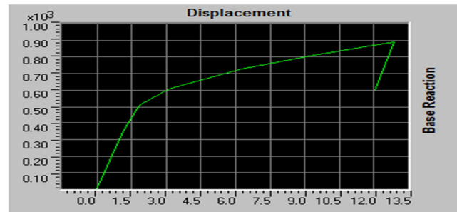
Fig-7, Case-2, Pushover curve for Displacement and base shear(Y-direction)
